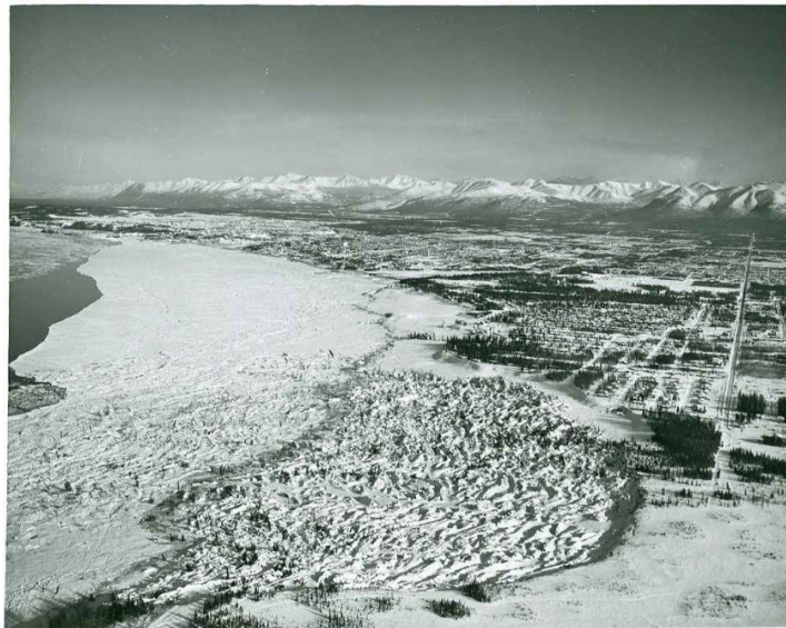
Figura 5: Lateral Spreading, Alaska 1964. (University Of Alaska Fairbanks, 2022)
