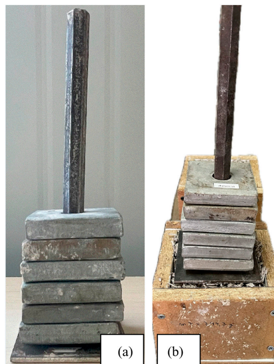
Figure 5. (a) Compacting device; (b) compaction of specimens.
